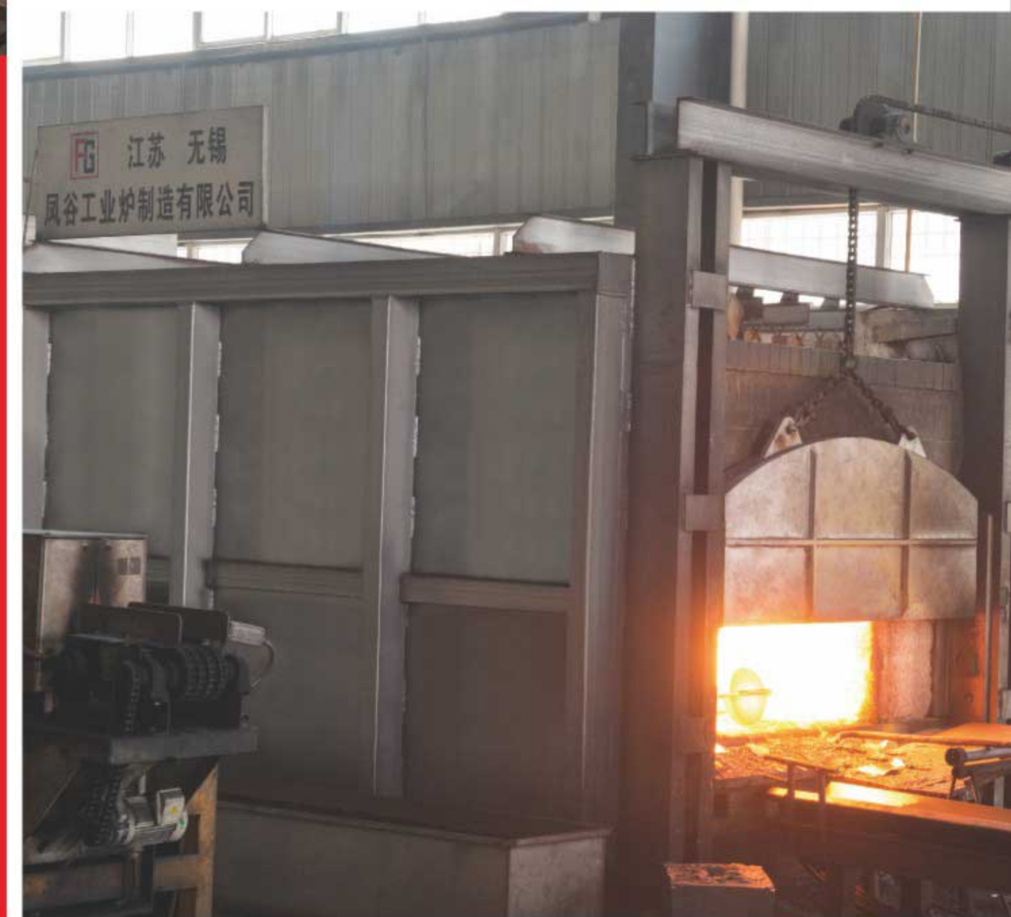
天然气加热(30t/天) Natural gas heating (30t/day)
